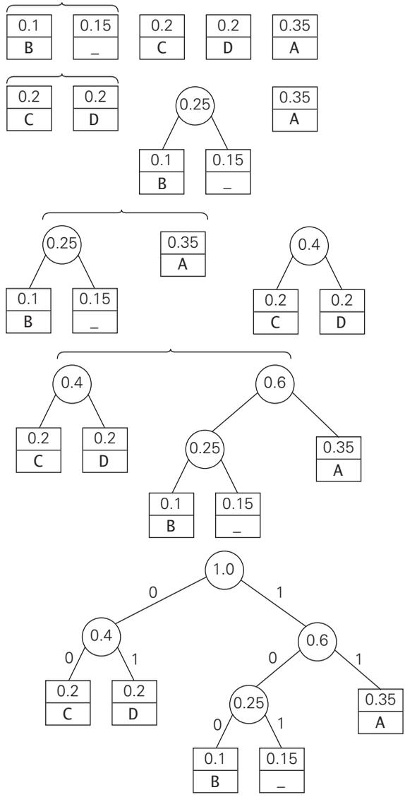
**FIGURE 9.12** Example of constructing a Huffman coding tree.
