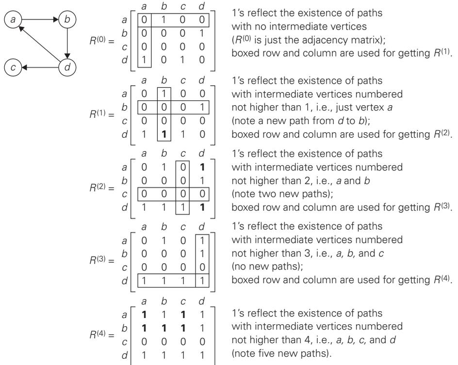
**FIGURE 8.13** Application of Warshall's algorithm to the digraph shown. New 1's are in bold.
