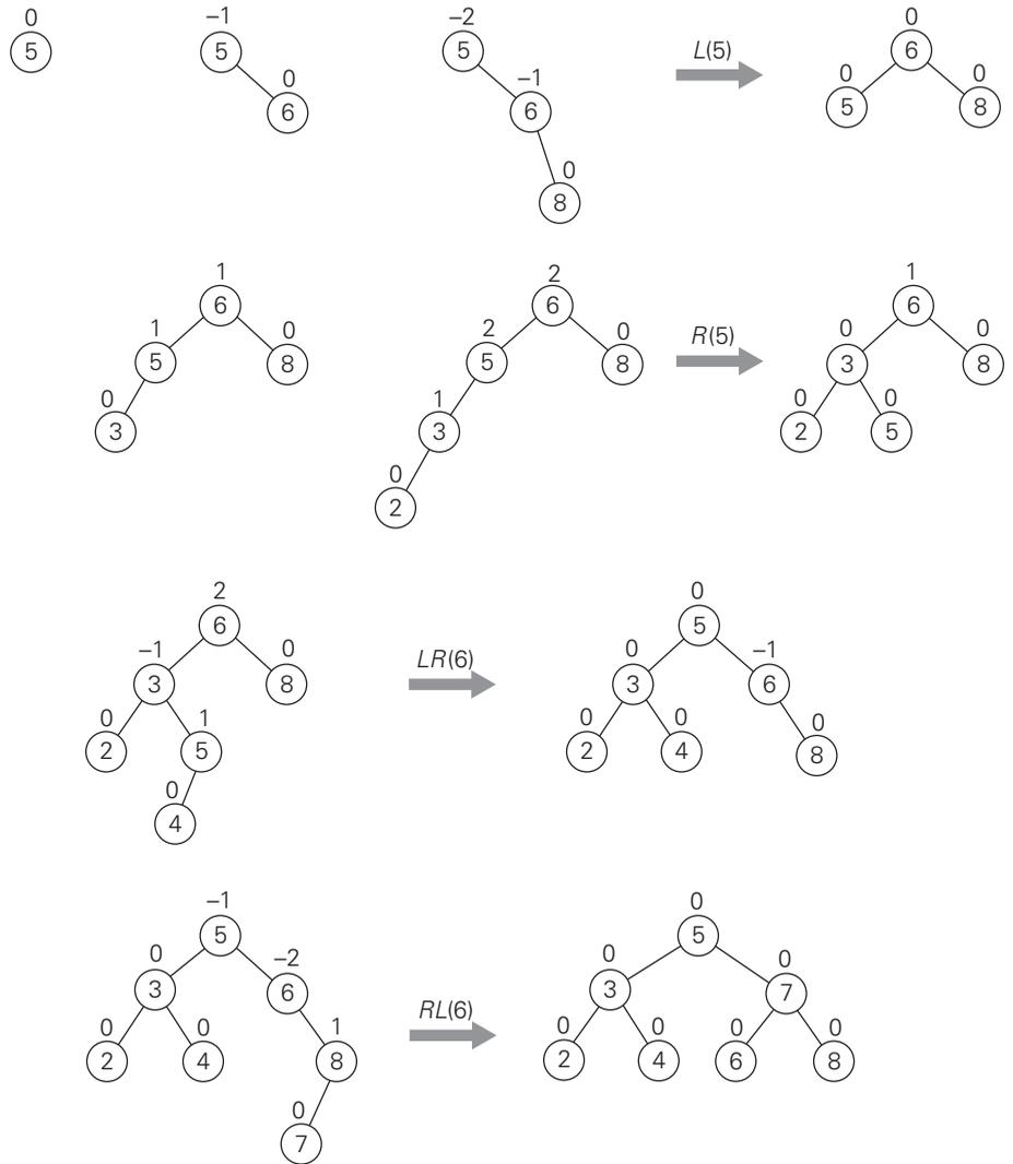
**FIGURE 6.6** Construction of an AVL tree for the list 5, 6, 8, 3, 2, 4, 7 by successive insertions. The parenthesized number of a rotation’s abbreviation indicates the root of the tree being reorganized.
