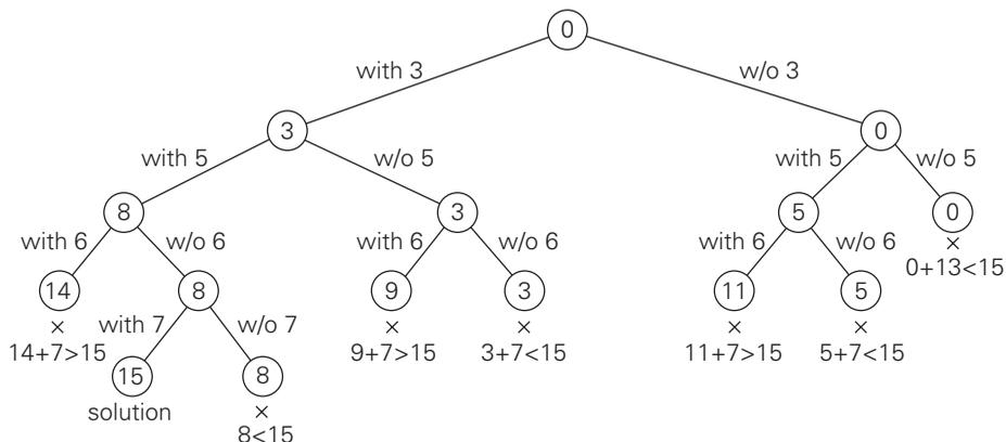
**FIGURE 12.4** Complete state-space tree of the backtracking algorithm applied to the instance  $A = \{3, 5, 6, 7\}$  and  $d = 15$  of the subset-sum problem. The number inside a node is the sum of the elements already included in the subsets represented by the node. The inequality below a leaf indicates the reason for its termination.
