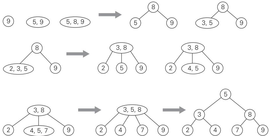
**FIGURE 6.8** Construction of a 2-3 tree for the list 9, 5, 8, 3, 2, 4, 7.
