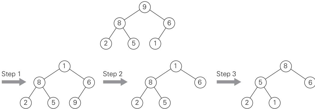
**FIGURE 6.13** Deleting the root's key from a heap. The key to be deleted is swapped with the last key after which the smaller tree is “heapified” by exchanging the new key in its root with the larger key in its children until the parental dominance requirement is satisfied.
