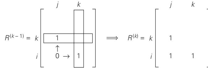
**FIGURE 8.12** Rule for changing zeros in Warshall’s algorithm.
