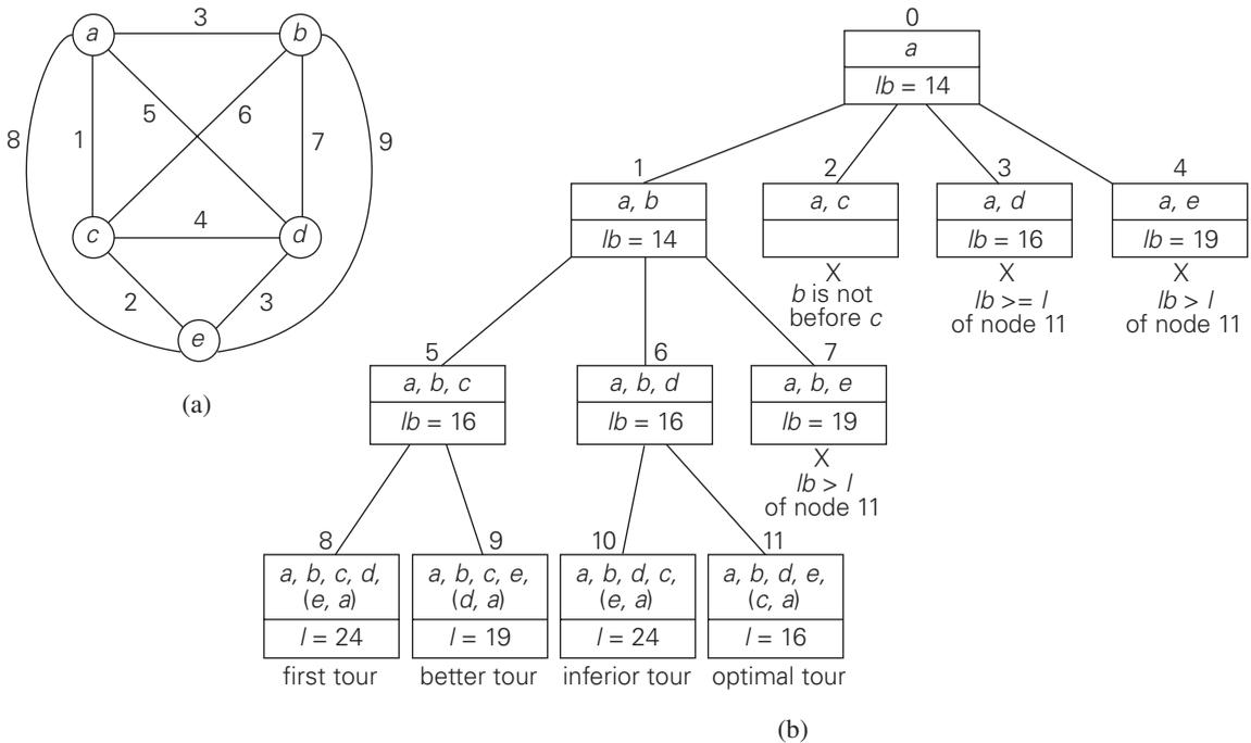
**FIGURE 12.9** (a) Weighted graph. (b) State-space tree of the branch-and-bound algorithm to find a shortest Hamiltonian circuit in this graph. The list of vertices in a node specifies a beginning part of the Hamiltonian circuits represented by the node.
