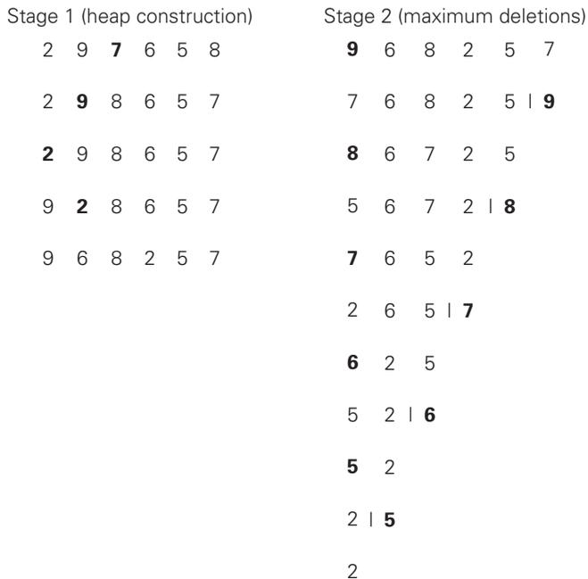
**FIGURE 6.14** Sorting the array 2, 9, 7, 6, 5, 8 by heapsort.
