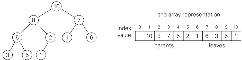
**FIGURE 6.10** Heap and its array representation.
