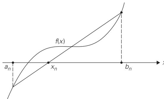
**FIGURE 12.20** Iteration of the method of false position.
