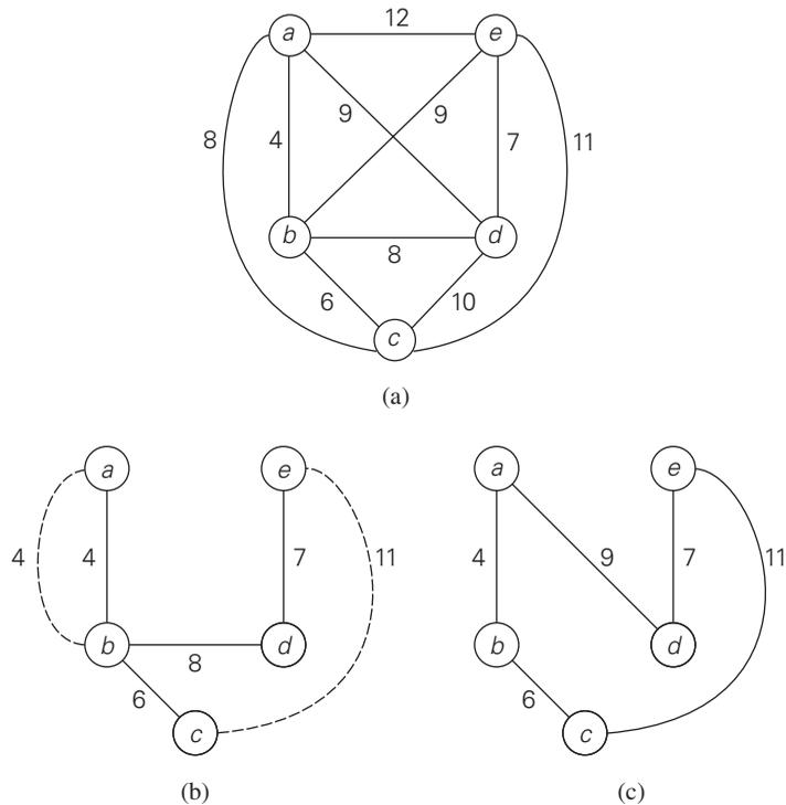
**FIGURE 12.12** Application of the Christofides algorithm. (a) Graph. (b) Minimum spanning tree with added edges (in dash) of a minimum-weight matching of all odd-degree vertices. (c) Hamiltonian circuit obtained.
