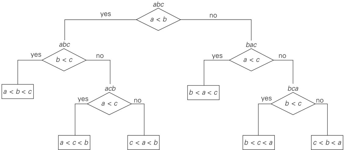
**FIGURE 11.3** Decision tree for the three-element insertion sort.
