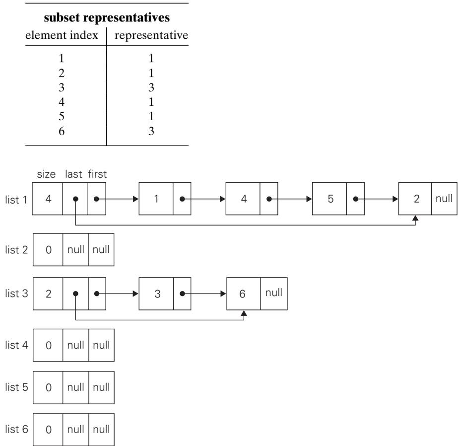
**FIGURE 9.7** Linked-list representation of subsets  $\{1, 4, 5, 2\}$  and  $\{3, 6\}$  obtained by quick find after performing  $\text{union}(1, 4)$ ,  $\text{union}(5, 2)$ ,  $\text{union}(4, 5)$ , and  $\text{union}(3, 6)$ . The lists of size 0 are considered deleted from the collection.
