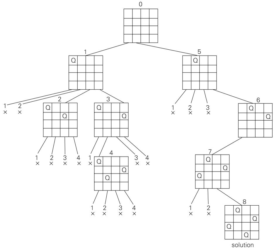
**FIGURE 12.2** State-space tree of solving the four-queens problem by backtracking.  $\times$  denotes an unsuccessful attempt to place a queen in the indicated column. The numbers above the nodes indicate the order in which the nodes are generated.
