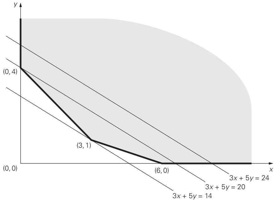
**FIGURE 10.3** Unbounded feasible region of a linear programming problem with constraints  $x + y \geq 4$ ,  $x + 3y \geq 6$ ,  $x \geq 0$ ,  $y \geq 0$ , and three level lines of the function  $3x + 5y$ .
