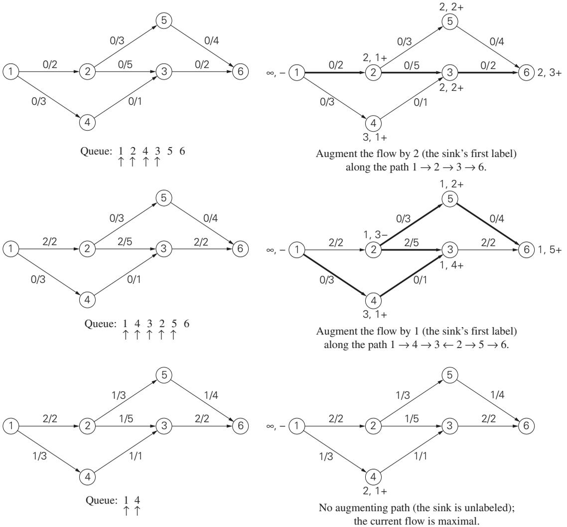
**FIGURE 10.7** Illustration of the shortest-augmenting-path algorithm. The diagrams on the left show the current flow before the next iteration begins; the diagrams on the right show the results of the vertex labeling on that iteration, the augmenting path found (in bold), and the flow before its augmentation. Vertices deleted from the queue are indicated by the ↑ symbol.
