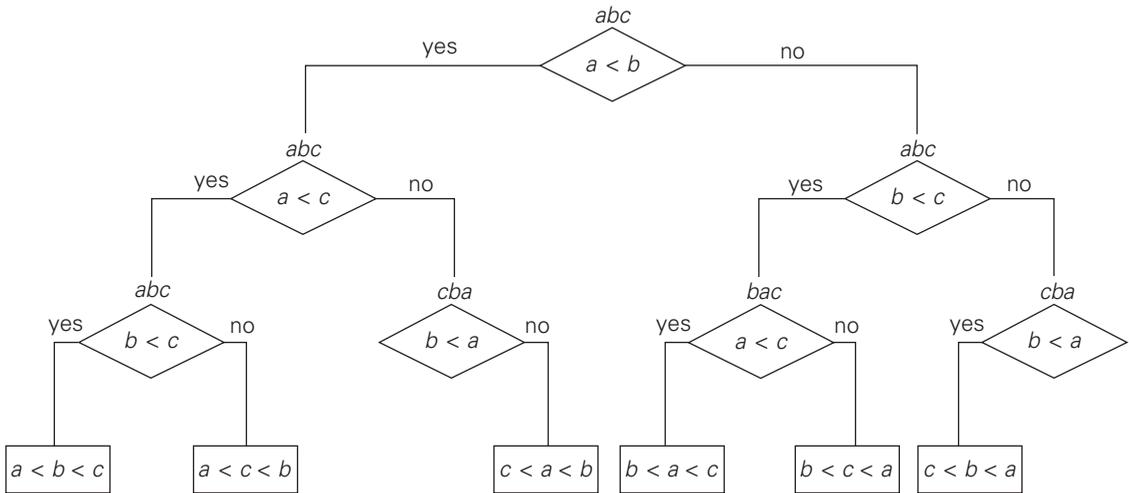
**FIGURE 11.2** Decision tree for the tree-element selection sort. A triple above a node indicates the state of the array being sorted. Note two redundant comparisons  $b < a$  with a single possible outcome because of the results of some previously made comparisons.
