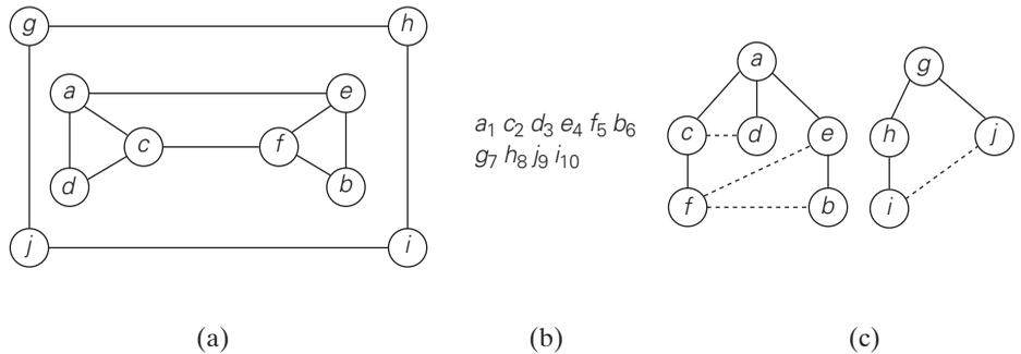
**FIGURE 3.11** Example of a BFS traversal. (a) Graph. (b) Traversal queue, with the numbers indicating the order in which the vertices are visited, i.e., added to (and removed from) the queue. (c) BFS forest with the tree and cross edges shown with solid and dotted lines, respectively.
