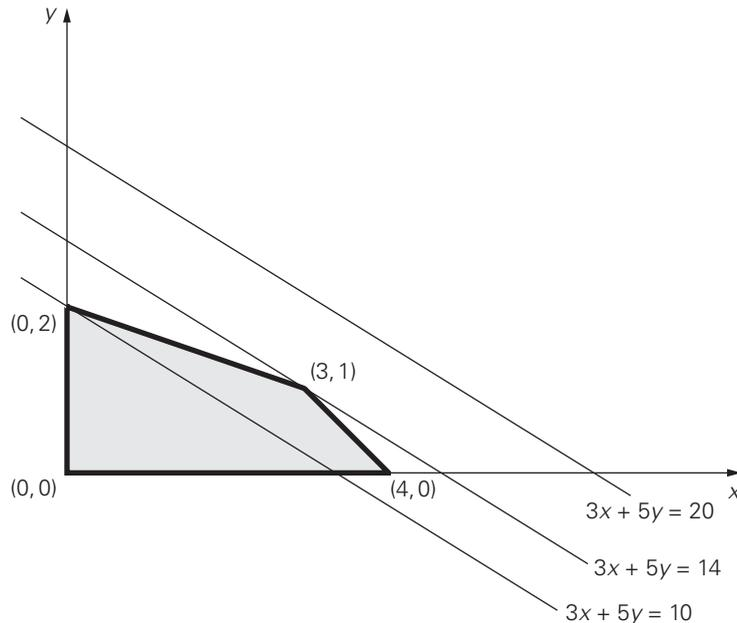
**FIGURE 10.2** Solving a two-dimensional linear programming problem geometrically.
