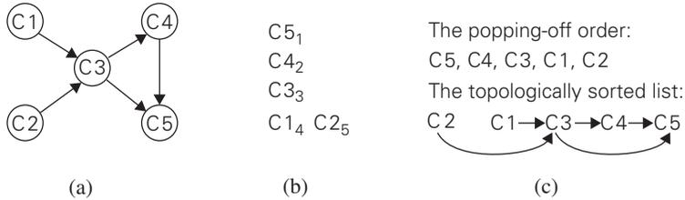
**FIGURE 4.7** (a) Digraph for which the topological sorting problem needs to be solved. (b) DFS traversal stack with the subscript numbers indicating the popping-off order. (c) Solution to the problem.
