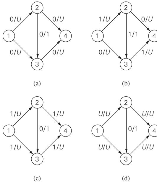
**FIGURE 10.6** Efficiency degradation of the augmenting-path method.
